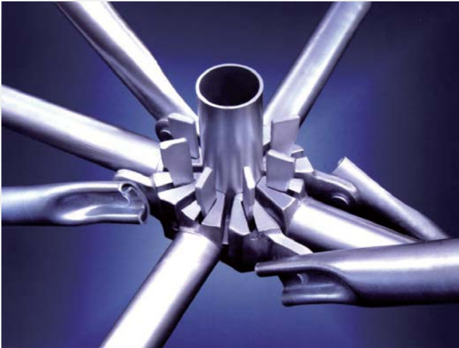
8 holes in one ring: Big hole: for Diagonal, Level Diagonal Small hole: for Horizontal
